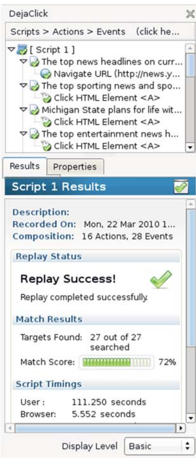
Above: DéjàClick sidebar shows real-time replay progress and summarizes match results, timings and network activity.
